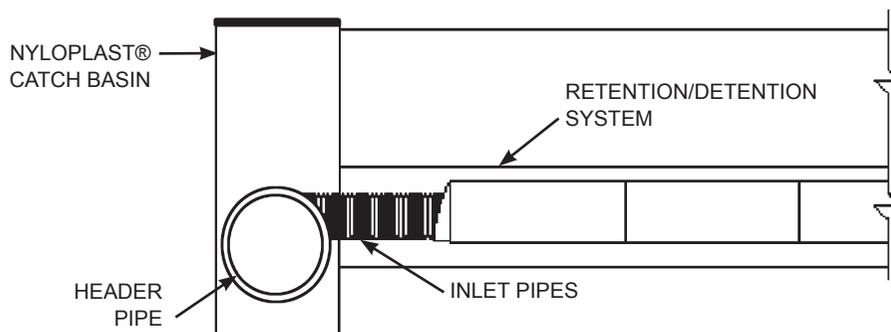
*The “eccentric header” is installed with its invert lower than the inlet pipes, thus acting as a sump to collect suspended sediment.*
